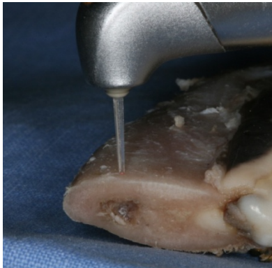
Fig. 2. Laser pre-drilling with Waterlase MD
