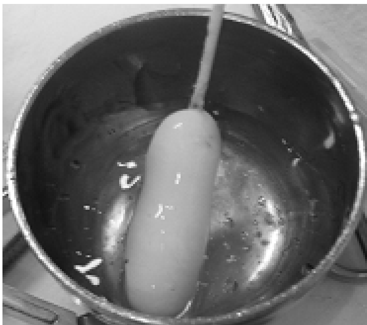
Fig. 2. Iceball formation of 17G cryoneedle in normal saline.
