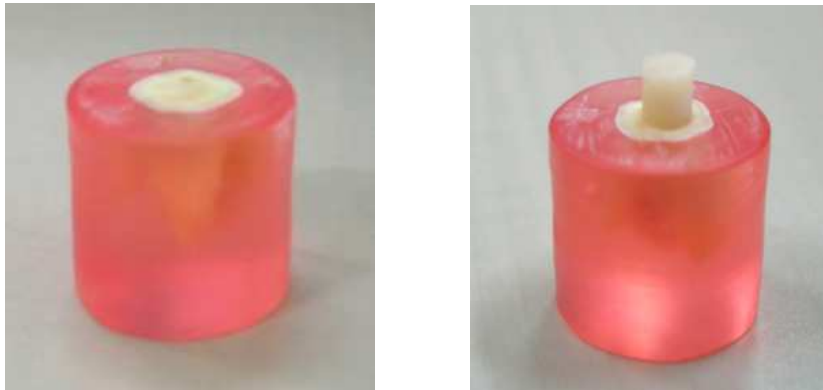
Fig. 4. Samples for the measurement of bonding strength.
