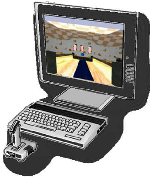
Figure 3. Hardware of virtual radial arm maze system. An IBM-compatible computer with color monitor was used for testing. Participants navigated through the mazes by manipulating a joystick. A speaker connected to the computer was used to provide auditory reward to the participants.
