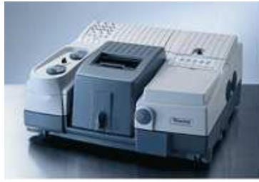
Figure 8. Equipment for surface composition analysis of impression materials (NICOLET 6700, Thermo Fisher Scientific, Waltham, MA, U.S.A.).
