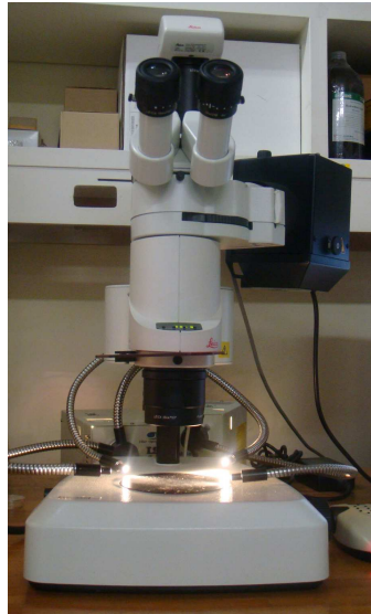
Figure 4. Equipment for observation of detail reproduction and compatibility with gypsum (Leica MZ16 FA, Wetzlar, Germany).
