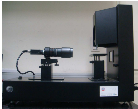
Figure 2. Equipment for contact angle measurement (Phoenix 300, SEO Co., Suwon, Korea).
