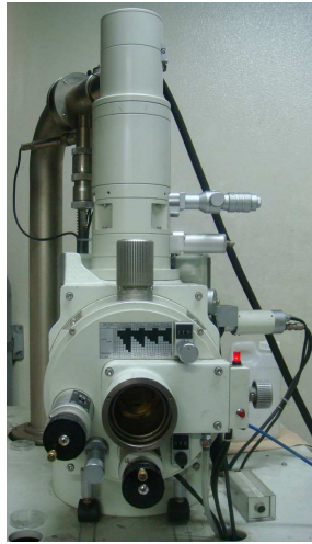
Figure 7. Scanning electron microscope (JEOL JSM-840A, Tokyo, Japan).
