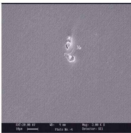
(c) NaF 2 % filled sealant( \times 3000 ).
