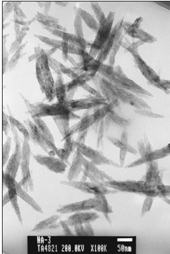
Figure 4. TEM image of HA nanoparticles.
