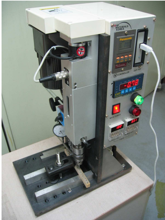
Fig 2. Photo image and schematic diagram of torque tester. ( Biomaterials Korea Inc. Seoul, Korea )
