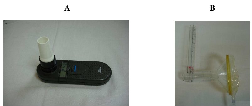
Fig. 2. Measurement of forced vital capacity and peak cough. A, Microspirometer for measurement of vital capacity . B, ASSESS for measurement of peak cough flow.
