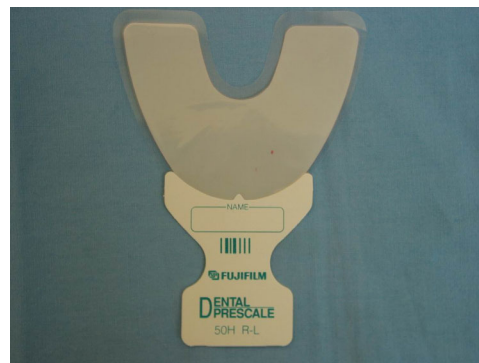
Figure 1. Dental Prescale® film (50H type-R, large size)
