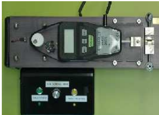
Fig. 5. Micro tensile tester used in this experiment
