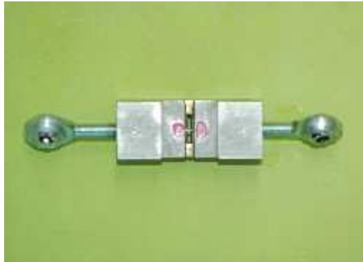
Fig. 6. Beam-shaped specimen attached on micro tensile device with Zapit(DVA, Corona, CA, USA)
