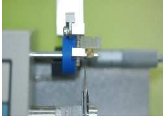
Fig. 4. Sectioning specimen attached on sectioning block with Metsaw™ (Topmet, Daejeon, Korea)
