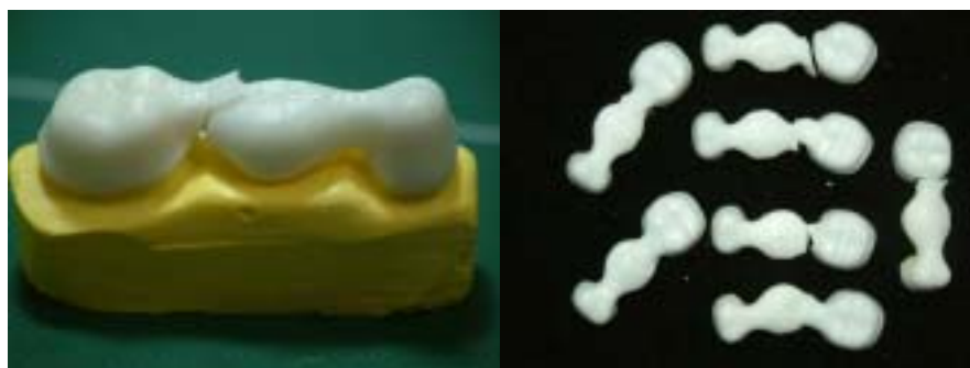
Fig. 7. Zirconia core has been fractured between pontic and second molar.
