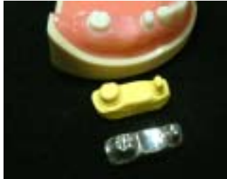
Fig. 1. Dies prepared for comparing fracture load of zirconia core for posterior fixed partial denture.
