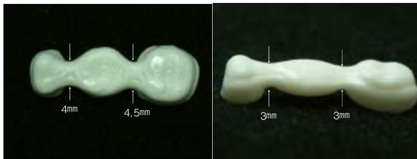
Fig. 2. Zirconia core constructed by CAD/CAM for posterior fixed partial denture. (occlusal view and lingual view)
