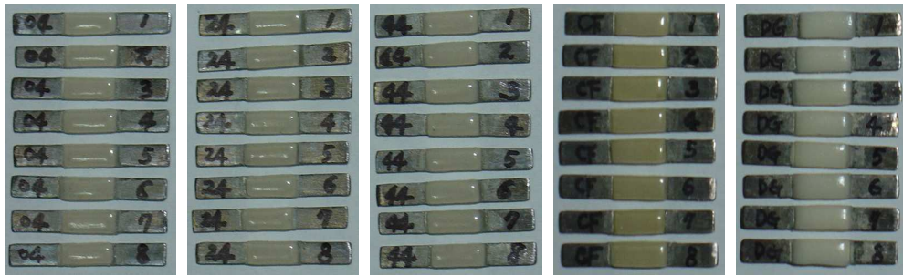
Fig. 9. Specimens for bond strength test.
