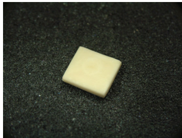
Fig 1. Ceramic block (10×10×2mm) prepared for surface treatments and bonding with composite resin
