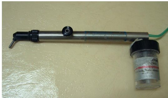
Fig 3. Microetcher (Danville Engineering, San Ramon, CA, USA): Instrument connected to the dental unit for intraoral air-abrasion
