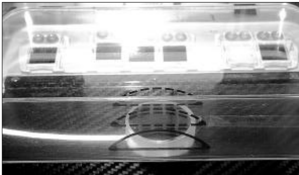
Fig. 1. A dosimeter was located just below the compression device, using the same conditions as, used for the digital measurement of compressed breast thickness, applied compression force, mAs and tube voltage, and entrance skin exposure was measured.
