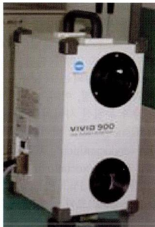
**Fig 2.** Vivid 900 (Minolta, Tokyo, Japan) laser scanner.
