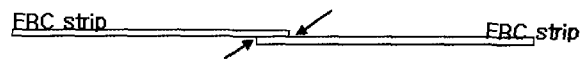
Fig 6. Critical section, the arrows indicate sudden changes in thickness of the FRC specimen.
