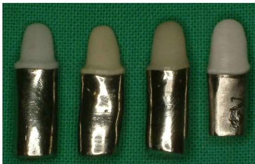
Fig. 3. Frontal view of the 4 cores and measurement dies. From left, Kavo Everest, Dent. solution, 3M Lava and Cerasys zirconia cores.
