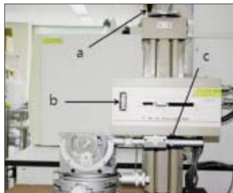
Fig. 1. Profilometer (a. vertical movement handle, b. set meter, c. rolling leg, d. stylus, e. fixation jig)
