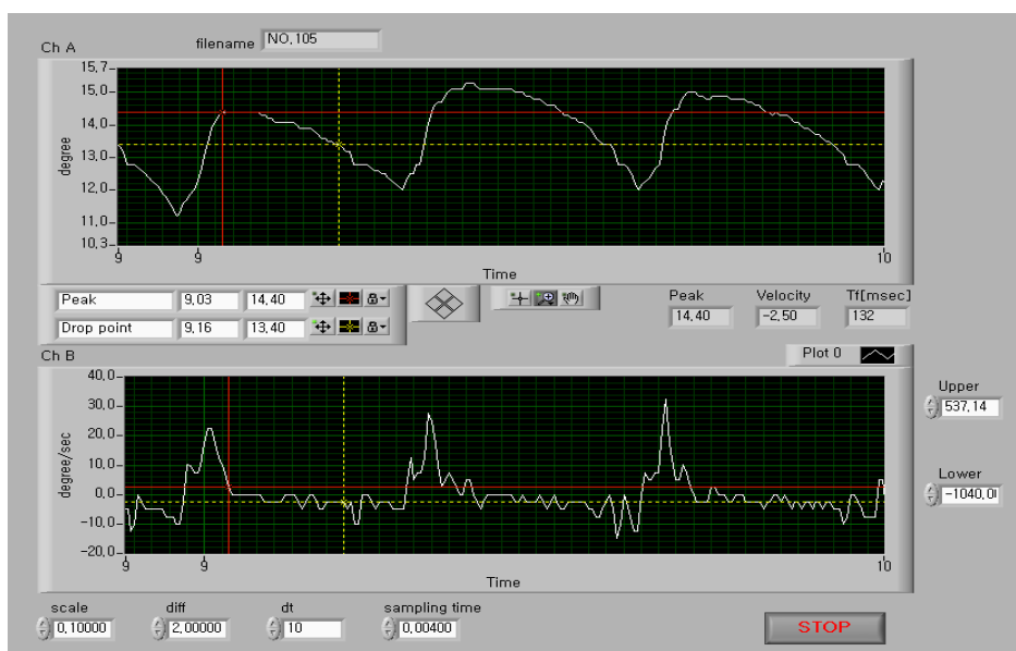
Figure 1. An eye tracing of a 42-year-old male diagnosed with infantile nystagmus shown with our program. Upper graph (Ch A) shows eye positional tracing and lower graph (Ch B) shows eye velocity tracing. Upward deflection denotes rightward direction. First, using cursors (red cross and yellow cross shown on the graph), we identified the interval of \pm 4^\circ/\text{sec} velocity. Second, we check the chosen velocity interval meets the \pm 0.5^\circ positional criterion. If the interval meets two criteria, we calculate foveation time (Tf) and standard deviation of position (SDp). For details, see the text.
