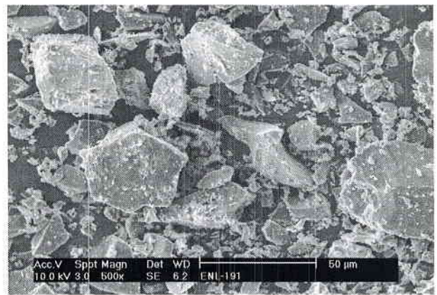
Fig. 9. FE-SEM image of veneer porcelain sample.
