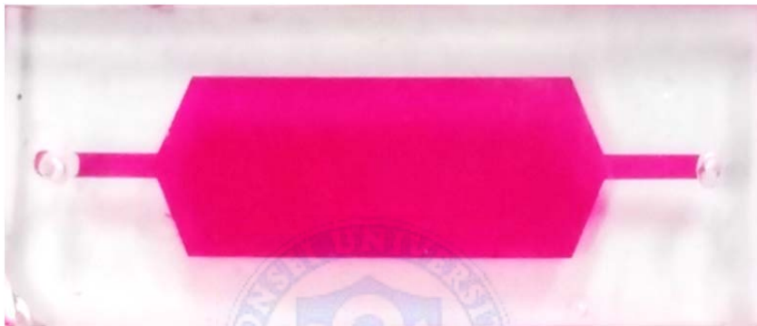
Figure 3.4. An overview of the cell chip. The cell chip has simple straight microfluidic chamber and two punched reservoirs.
