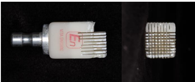
Figure 1. A PICN-resin specimen was cut by a diamond saw.
