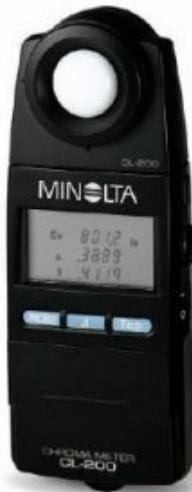
**Fig. 3** Chromameter for measuring the luminous intensity and the color temperature (CL-200, Minolta Corporation, Osaka, Japan)
