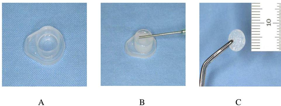
Figure 1. Cylinder type mold (8mm in diameter) used in this study (A). For peripheral seal, additional solution was injected into the block margin (B). The final disc-shaped implant was 3 mm in height and 8 mm in diameter (C).
